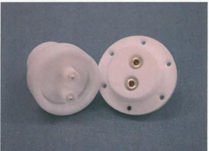
■ Coaxial connector of face contact
